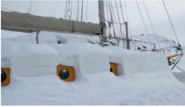
A snow cover with opening built over the portholes to let in light.
